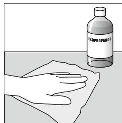
1. The surface must be dry, free from dust, oil, oxides, parting agents and other impurities. The surface to be glued should be cleaned using a clean cloth and isopropanol / water (50/50). When using other appropriate cleaning agents, ensure that they do not attack the surface nor leave any residues.
