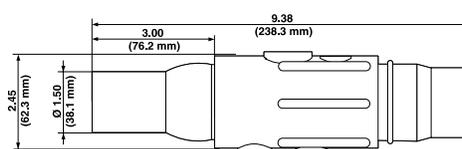
Ball Nose In-line Latching Female Connectors - Crimped
