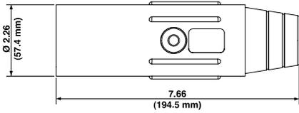
Ball Nose In-line Latching Male Connectors S-Series
