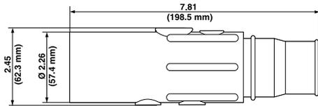
Ball Nose In-line Latching Male Connectors - Crimped
