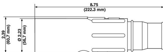
Taper Nose In-line Latching Male Connectors - Crimped
