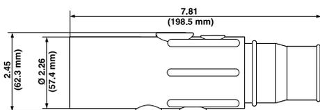
Ball Nose In-line Latching Male Connectors - Crimped
