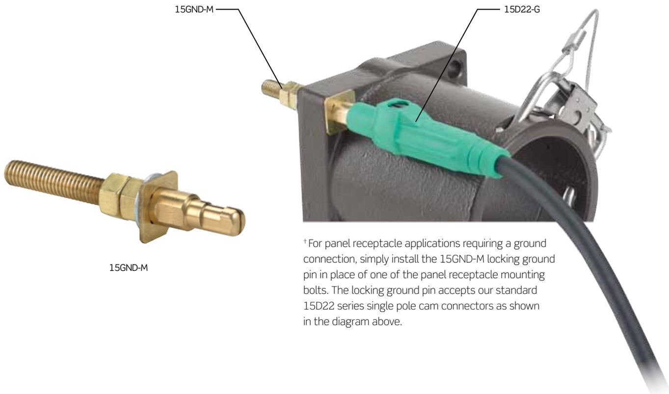
† For panel receptacle applications requiring a ground connection, simply install the 15GND-M locking ground pin in place of one of the panel receptacle mounting bolts. The locking ground pin accepts our standard 15D22 series single pole cam connectors as shown in the diagram above.
