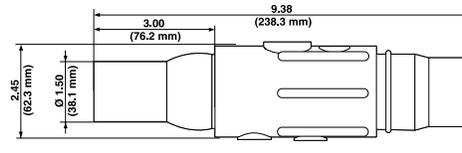
Ball Nose In-line Latching Female Connectors - Crimped
