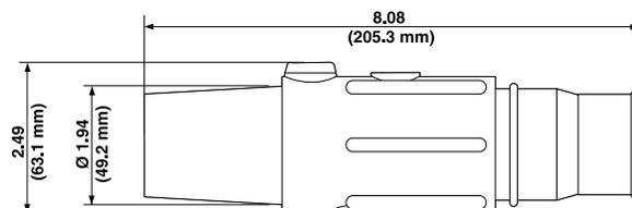
Taper Nose In-line Latching Female Connectors - Crimped
