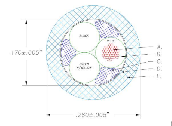
18 GAUGE 41x34BC BUNCHED 15 MILS PVC INSULATION 105°C 300V 13 MILS MIN. PVC INSULATION
