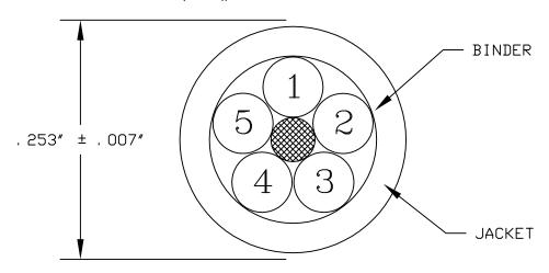
COMPONENTS - SINGLE CONDUCTOR #20AWG (SC#20)
