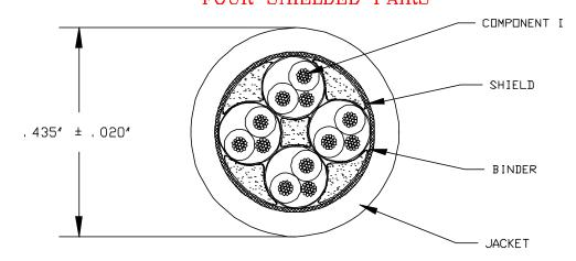
COMPONENT I -TWISTED PAIR SHIELDED #22 AWG (TPS#22)
