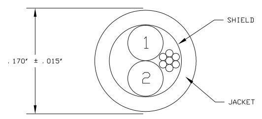
COMPONENT I- CONDUCTOR: #24AWG 19/36 TINNED COPPER
