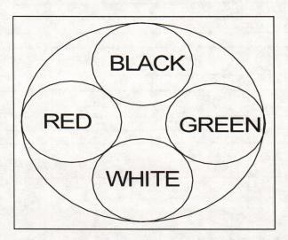
THE FLEXIBILITY OF THIS WIRE IS IMPORTANT TO THE SPECIFIC USER'S REQUIREMENTS. THE BENDING RADIUS SHOULD BE 8 TIMES OR LESS THE CABLE OUTSIDE DIAMETER. THIS RESULTS IN A BENDING RADIUS OF 1.34 INCHES OR LESS. THE MORE FLEXIBLE THE BETTER.
