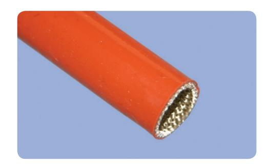
**GES** is a braided fiberglass sleeve with a silicone rubber coating designed to provide electrical insulation. The thickness of the silicone coating determines the dielectric strength, which ranges from 4 to 10 kV.
