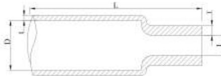
It is widely used in the fields of electricity, communication, automotive for connection insulation and rust-proof of metallic product.
