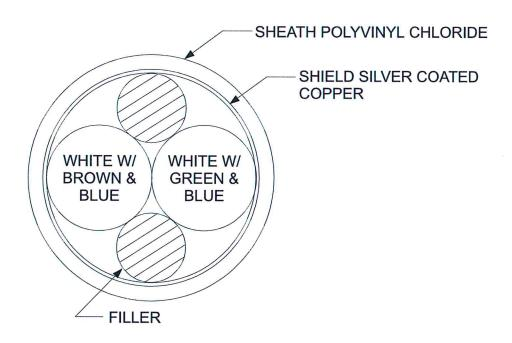
FIGURE 1. Cable configuration.
