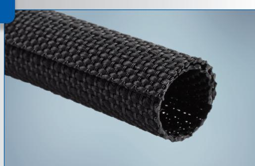
TwistWrap™ 2403 is a self-wrapping sleeve designed to enable fast and easy wire harness bundling. Woven of both monofilament and multifilament polyester yarns theproduct is both flexible and lightweight. The polyester construction eliminates problems associated with trapped heat and humidity and also eliminates operator skin irritationduring assembly. The combination of materials also enables the product to provide a level of abrasion protection for the wire bundle.
