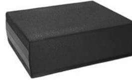
These deluxe instrument cases feature separate front and back panels, internal slots to hold PC boards in place and internal mounting posts for securing PC boards. Case has metal studs for non stripping of screws holding the case together. Front & back panels are plastic and are easily machined and drilled. PB250 has grey case top and front & panels are black. PB200 is all black.
