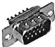
Hi-density types pack more contacts into the standard D-sub configuration. Solder cups are tinned for soldering. Contact areas are gold plated, resist corrosion. Steel shells and glass-fiber reinforced plastic insulator (UL94-V-0).
