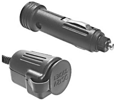
A 10 ft. extension cable with fused 12V cigarette lighter plug on one end to 12V socket with dust cover. 18 AWG wire with 2A fuse.
