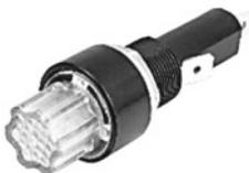
Rating 20A 32V DC, holds 1/4"-1-1/4" 3AG type fuse. Can be used in panel up to 3/8" thick, mounts in .63" (16.0mm) mounting hole 94V UL material, LED indicates when fuse is blown.
