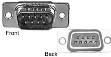
Solder cup contacts are tinned for positive soldering of wire. Contact areas are gold plated. Steel shell with glass-fiber reinforced plastic insulators (UL94V-0).
