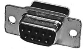
Male shell indents assure positive contact, firm grip to mating female. Crimp contacts are precision formed brass; contact areas are gold plated and crimp areas are tinned. Typically used with 24 or 22 gauge wire.
