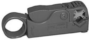
The cutters are easily adjusted for non-standard cables by turning two set screws using the hex wrench stored in the handle. After the cable is cut, it is automatically stripped in a single action by removing the tool from the cable. Spare cutting blades are available and are readily installed.
