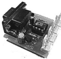
No external power is required. The data stream is easily logged and processed. You must use a terminal program set at 2400 baud, 8 bits, no parity and 1 or 2 stopbits. Information is given about a free Term.exe program that you can download from our associates web site.
