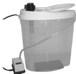
This handy etching tank system will handle P.C. boards up to 8" x 9" and 2 at a time. The tank holds 1.35 gallons of etching solution. The system is supplied with air pump for etchant agitation, heater for keeping etchant at optimum temperature and convenient board holder. Tank has tight fitting top to prevent evaporation when not in use.
