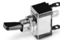
This is a SPST, ON-OFF switch and designed for use at automotive (12-14V DC) voltages: rated at 30 amps. This is a popular new look in actuator styles. The handle (actuator) is Black and tipped with an LED; three color choices. The LED will draw only 20 mA at normal automotive voltages. Mounting hole diameter: 1/2" Terminals will accept 1/4" push-on solderless connectors or may be soldered.
