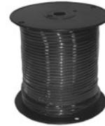
Bulk "S-Video" cable for making your own cables in whatever lengths needed. Use with Philmore connectors Nos. EMA4 and 45-106G etc.. The cable has a black PVC outer insulation, red and white inner conductors (two) that have insulated shields for a total of four conductors. Supplied on spools.
