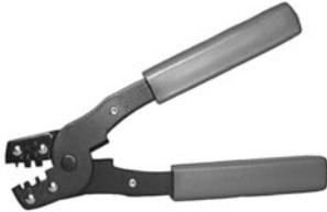
Hand held tool crimps D-Sub pins (male and female) with a single squeeze on the contact material. Has built-in wire cutter.
