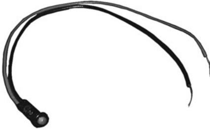
Sub-miniature snap-in panel lamps press-fit into a 0.173" diameter hole. Uses the industry standard T1 size LED. Lead wires are 6" long, (26 Ga.), stripped .380" on ends (red and black insulation indicates polarity). The 2 volt values are regular LED's, use a resistor for voltages that are higher than 2 volts; package includes "how to" calculate resistor values.
