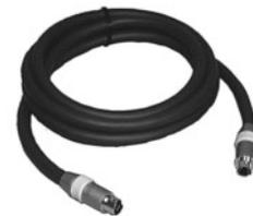
Bulk cable user information: Cable is comprised of two fully shielded (1 red and 1 yellow) 75 ohm coaxial cable. Coaxial cable outside diameter .122", inner insulator is PE foam .087 O.D. (24 awg stranded center conductor) with a nominal capacitance of 16.9 picofarads per foot. Shield is copper braid woven for 95% coverage. Total cable O.D. is .315" outer insulation dark grey in color.
