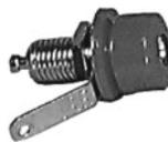
.175", accepts standard banana plugs. Jack mounts in 5/16" dia. hole (or use 1/4" when jack will ground to panel) in panels up to 3/8" thick. Insulator and head is polycarbonate, body is nickel plated brass.
