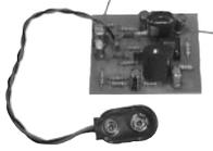
Today amplifiers are designed for flat response and they make the old phonograph recordings sound very flat. Using an RIAA preamplifier compensates for today's flat amplifiers exactly as the old phonographs were able to do. This kit duplicates the RIAA curve accurately; at a kit price. Operation on 9 to 12 V. DC.
