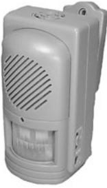
This entry alarm allows user to play recorded message upon sensor interruption. Recordable message length is about 20 seconds. Detection area up to a distance of 20 feet with a radius of 100 degrees. Supplied with mounting bracket that allows 120 degrees swivel adjustment. Powered by (4) AA batteries (not included). External jack: 6V 600mA regulated DC adaptor (not included) or 3-4.5V 500mA non-regulated DC adaptor (not included).
