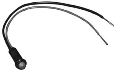
2 Volt LED Panel Lamp for 1/4" hole size. Considered the "universal" type as it can be used with virtually any DC voltage with a resistor (package shows how to determine resistor value). And it can be used with AC voltages with a diode and resistor. The lamp has 6" long wire lead set (black / red), which is stripped and tinned, ready to solder. Body color black (nylon).
