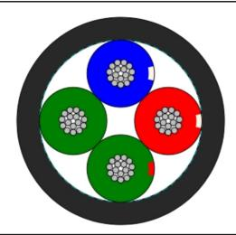
**Components** Four 18 AWG, PVC Insulated Conductors
