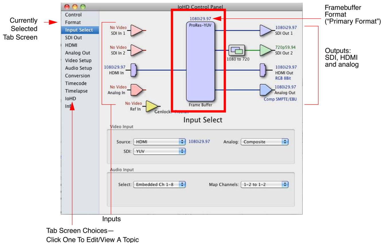
**Framebuffer**—the framebuffer is the “engine” in the Io HD where active video operations take place using Final Cut Pro, other 3rd-party applications, or even Io HD itself. The framebuffer has a format (called the “Primary Format” and color space that it follows, as defined in the Tabbed Windows or via external application software such as the “Easy Setups” in Final Cut).
