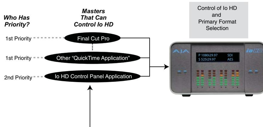
When you click in an application window, the “Master” controlling Io HD changes, possibly changing the Format Selections in effect. This happens because each application has its own sets of control parameters
