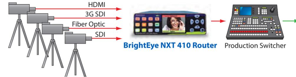
Add more inputs to your production switcher or master control switcher. Feed cameras and other SDI and HDMI sources to a BrightEye NXT 410 Router and take one or more of the router outputs into the production switcher or master control switcher. This is also a great way to integrate HDMI signals into an SDI workflow.
