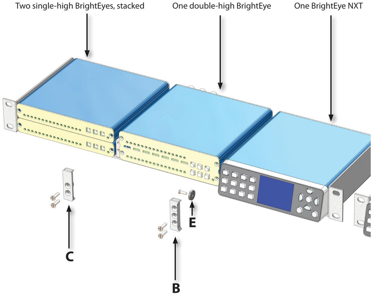
Illustration of BrightEyes and a BrightEye NXT installed in the rack mount, using a BrightEye to BrightEye front retainer (**C**), a BrightEye to NXT front retainer (**B**) and an NXT Retainer Washer (**E**), exploded view
