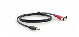
Kramer's A35M/2RAM and A35F/2RAM series cables are simple adapters which have a stereo 3.5mm connector at one end, and two male RCA connectors at the other. They provide passive conversion between 3.5mm and dual RCA connectors, most often adapting a PC sound card or MP3 player to the audio inputs of a sound system or display device.
