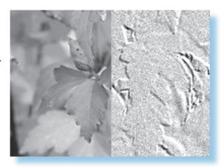
Split Screen displays the noise-reduced output next to the original scene.
