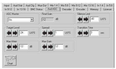
LevelTrack is controlled through Avenue PC where you can set your own audio automatic gain control target levels. Both 1770 algorithms and VU metering are provided.
