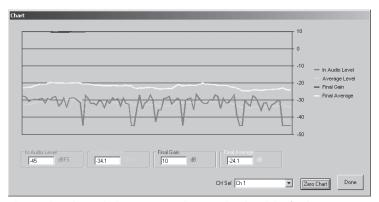
The LevelTrack graph shows your audio input level and the final gain applied to the audio signals.
