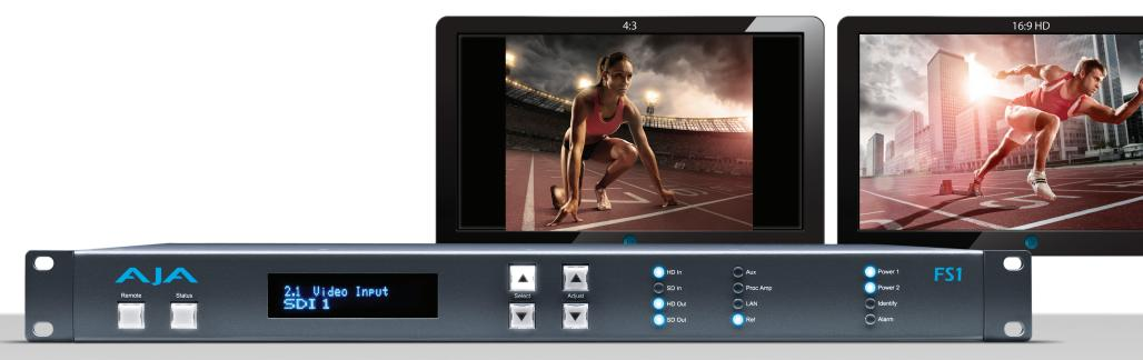
AJA's FS family of frame synchronizing converters deliver power and flexibility for up/down/ cross conversion in just 1RU of space. Align mismatched signal types, including computer DVI signals, to establish a consistent format for post production or broadcast.
