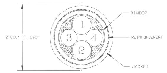
COMPONENT I - SINGLE CONDUCTOR #4/OAWG (SC#4/O)
