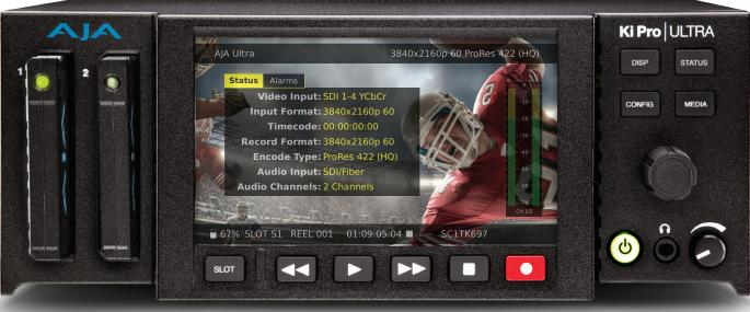
Ki Pro Ultra is a next generation 4K/UltraHD/2K/HD capable file-based video recorder and player with broad support for video formats and frame rates (up to 4K 60p) and flexible input and output connectivity, including 3G-SDI, Fiber and HDMI.
