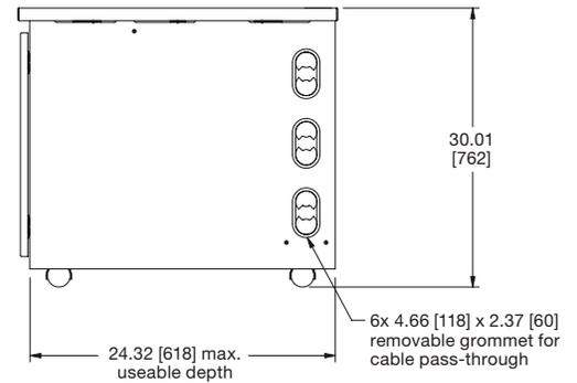
LD-1230\_\_\* side rack gangs to desk w/ included hardware and provides 12 rackspaces for equipment mounting behind an attractive smoked plexi front door. In order to join LD-1230\_\_\* side rack to LD wedges, the LD-WK joiner kit is required.
