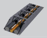
Use dividers horizontally and vertically to separate the track into separate cavities. Install just one cable per separated cavity. If absolutely necessary, two small or a small and a big cable can share a cavity.
