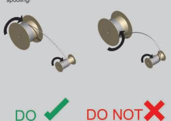
Ring put ups require careful uncoiling by rolling the ring upright over the floor.
