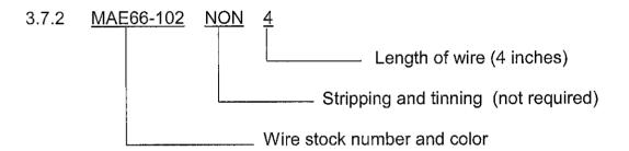
NOTE: On this example, the stripping and tinning are not required; this wire is cut to length only.
