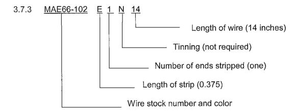
NOTE: On this example, the wire is cut to length, one end stripped but not tinned.
