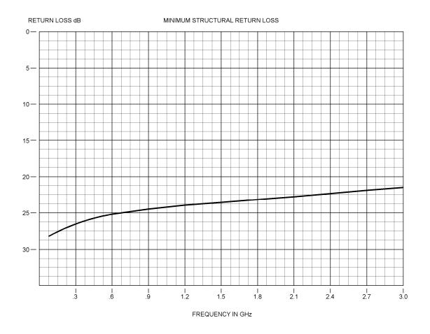
FIGURE 3. <u>Structural return loss</u>.
