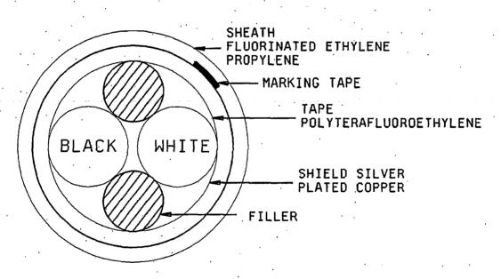
FIGURE 1. Cable configuration.
