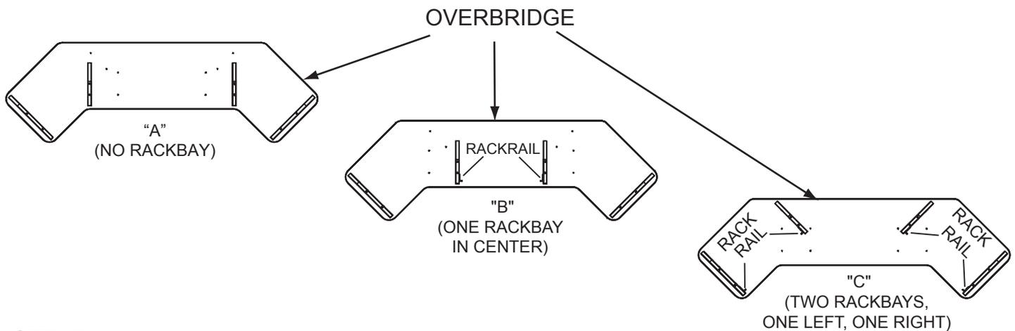
**NOTE:** Rackrail is a user installed option on "B" and "C" configurations.
