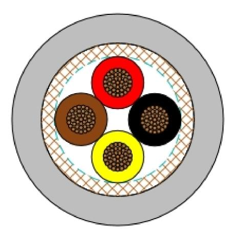
**Description:** Shielded Jacketed 4 Conductor Cable (28 AWG 40/44 TC, .006" PFA), 40 AWG TC BRD, .015" GRY PVC
