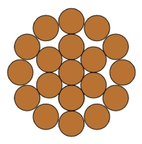
**Description:** Concentric Stranded Conductor 18 AWG 19/30 NPC
