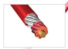
Construction features insulated bundles of Type 2 Litz wire twisted around a central fiber core with optional outer insulation.
