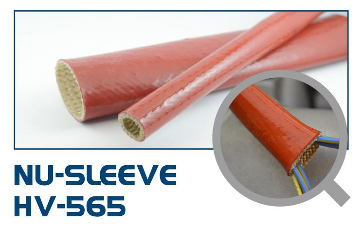
NU-SLEEVE HV-565 is a heavy wall coated fiberglass sleeving made by applying a heavy coating of liquid silicone rubber to a fully annealed fiberglass substrate. The HV-565 sleeving is extremely resistant to abrasion, offers better coating adhesion to the fiberglass compared to extruded type sleevings and has a high heat/flex capacity.
