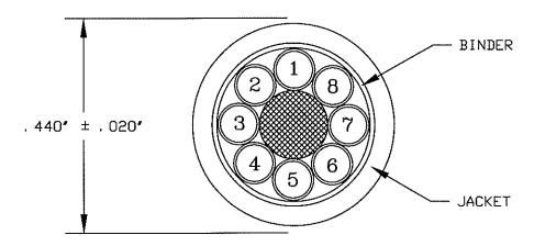
COMPONENT I -CONDUCTOR #18AWG 19/, 0092 BARE COPPER INSULATION: PVC-, 015' NOMINAL WALL (ITEMS 1-8)
