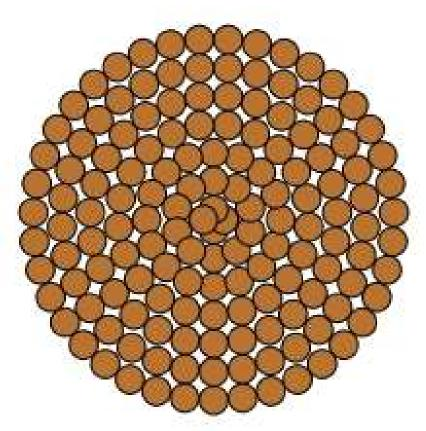
**Description:** Ropelay Stranded Conductor 2/0 AWG 5292/36 BC
