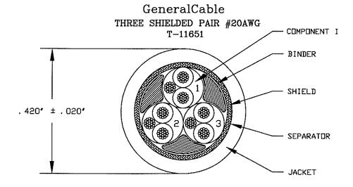
COMPONENT I - (ITEMS 1-3) TWISTED PAIR SHIELDED #20AWG (TPS #20) PRIMARY - CONDUCTOR: #20AWG 19/32 TINNED COPPER INSULATION: CROSS-LINKED POLYETHYLENE-, 016' NOMINAL WALL DIAMETER: .072' NOMINAL
