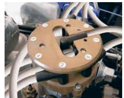
Insultherm Ultra-Flex is a highly flexible heat protection with no added coatings or binders
