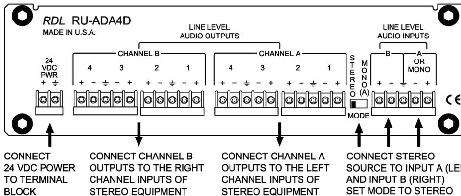
NOTE: IF THE MODE SWITCH IS SET TO MONO, THE MONO SOURCE WILL FEED ALL OUTPUTS. CONNECT EACH OUTPUT (CHANNEL A OR B) TO THE INPUT OF MONO EQUIPMENT
