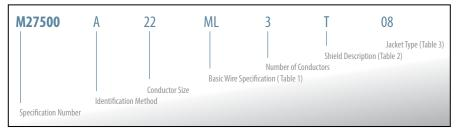
All the basic wire specifications listed below may be supplied by RSCC Aerospace & Defence as components in WC 27500 cables. These range from low temperature PVC/Nylon leads through high performance, high temperature constructions. The basic wire specification, part number designation symbol, and a brief description of the insulation type are listed in Table 1.
