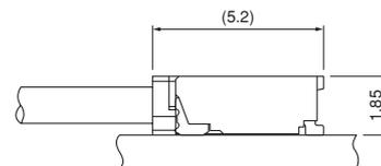
Note: 1. The above figure is the figure viewed from the connector mounting side.
