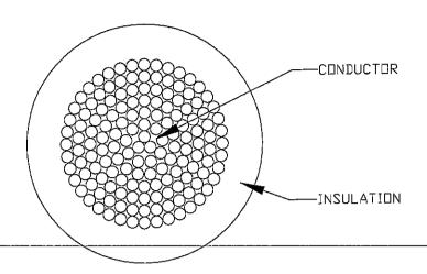
**NOMINAL DIAMETER** CONSTRUCTION: (1 REQUIRED) 1 AWG 225/24 Tinned Copper
