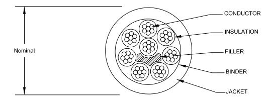
CONDUCTOR: #18AWG (7/w) Tinned Copper Class B Strand per ASTM B8, B33
