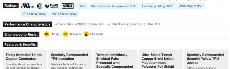
Offers superior first-line defense against tearing, abrasion, impact, oil, ozone, UV exposure, and most chemicals. Flame and heat resistant. Extreme all-weather flexibility.
