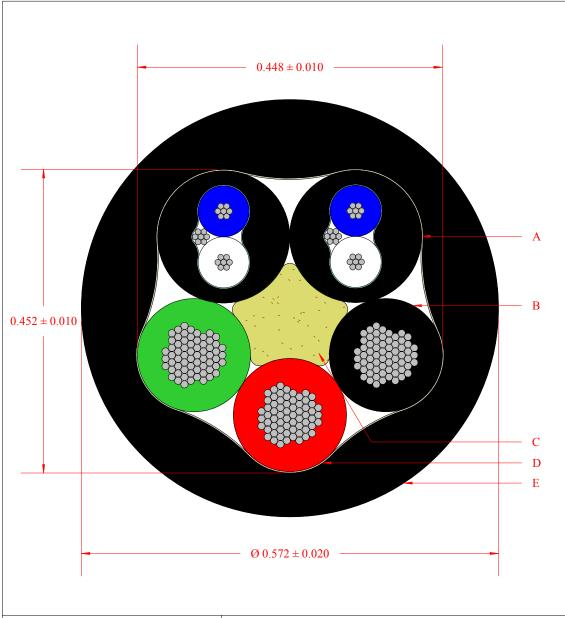
A: (2) 24 AWG 2C 7 Strands Tinned Copper Foam Polypropylene Insulated
