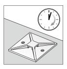
5. Depending on the type of adhesive, wait for several minutes (synthetic rubber) or hours (acrylate) so that the adhesive can bond completely with the surface.
