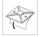
3. Peel off protective backing and ensure the adhesive area is not touched.
