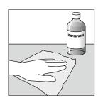
1. The surface must be dry, free from dust, oil, oxides, parting agents and other impurities. The surface to be glued should be cleaned using a clean cloth and isopropanol / water (50/50). When using other appropriate cleaning agents, ensure that they do not attack the surface nor leave any
