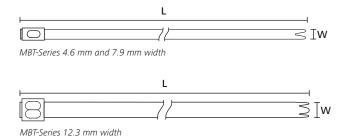
The MBT-Series (up to 7.9 mm) can be used in combination with the stainless steel P-Mount. The mount is simple to install with a screw or bolt and ensures a durable fixing solution. Please see page 143.
