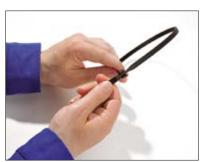
1. Insert the thin part of the cable tie into the open lock head.
