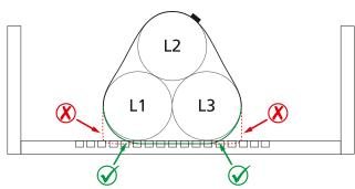
Best practice for installation in trefoil formation. Ties should be bundled as closely as possible to the cables for a smooth loop and to avoid sharp edges.
