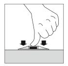
**4.** Press down firmly on the base with the thumbs for several seconds.
