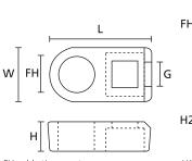
FH cable tie mounts (plan and side view)
