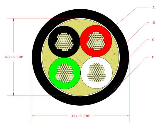
A: 12 AWG 4 Conductors 65 Strands Bare Copper with PVC Insulation Overall Polyvinylchloride Jacket
