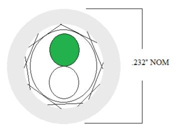
DESCRIPTION: TWO CONDUCTOR 16 AWG, PVC-NYLON, BRAID SHIELD,
