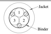
Components Three 18 AWG Insulated Conductors
