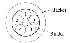
**Components** Five 18 AWG Insulated Conductors
