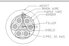
**Description:** 3/Pairs # 20 AWG; HD-PE Insulation, Each pair shielded, Overall Polyurethane Jacket.
