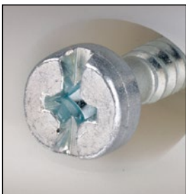
Shrouded pockets in cord clamp prevents slippage of screwdriver blade when tightening clamp screws.
